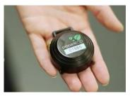
Radon is odourless, colourless and tasteless. To assess the level of radon in an existing building, specialist detectors must be placed in the property before being sent to a laboratory for analysis. Radon detectors are small and discreet, and the whole process including laboratory analysis is inexpensive. As radon levels fluctuate according to seasonal and occupational variances (e.g. amount of ventilation through opening windows), a three-month test period is
